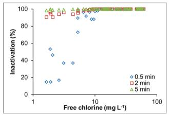
Figure 3. Inactivation of bacteria collected from aviary hen house treated with MLAEW at different free chlorine concentrations, and treatment time 0.5, 2 or 5 min
