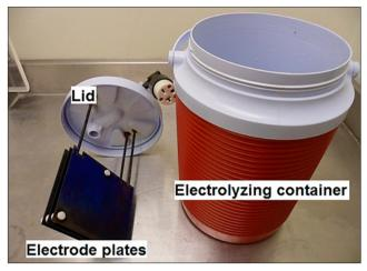
Figure 1. Electrolyzing container and components
